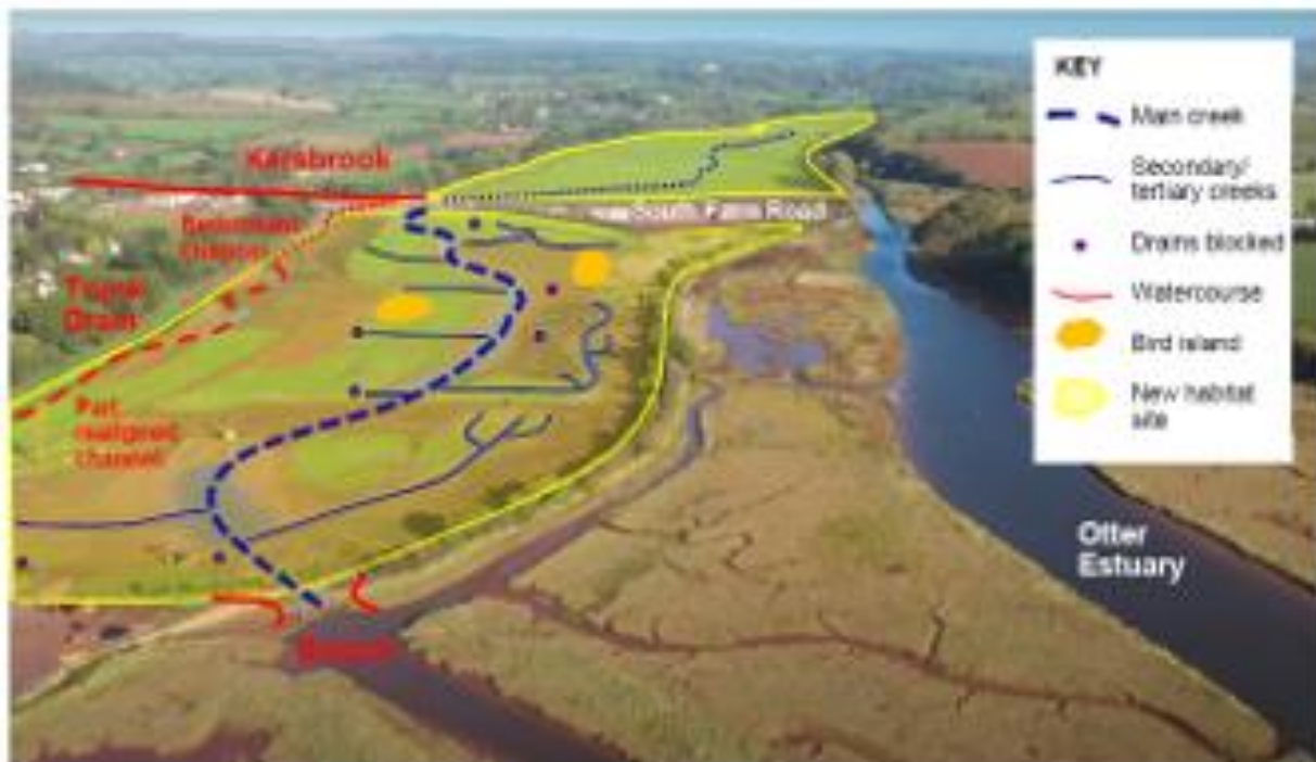
Figure 6.9 Creek network system at Big Marsh South. Source Jacobs
